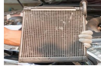
Fig. 9 Plate finned tube heat exchanger [21]
