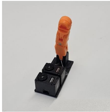
FIG 36: original single finger testing rig
