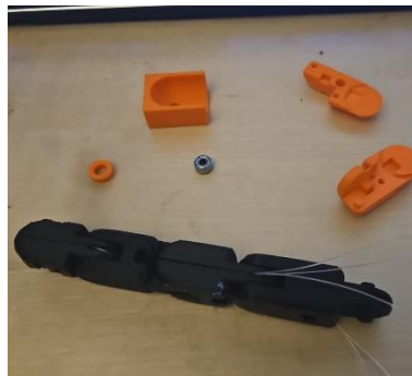
FIG 35: V4 single finger assembly and V4 tips and mould printed
