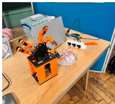
FIG 38: First full assembly including routing and V1 motor hub
