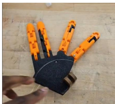
FIG 37: First full hand assembly including routed carpal
