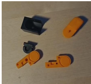
FIG 34: V4 tips and mould printed
