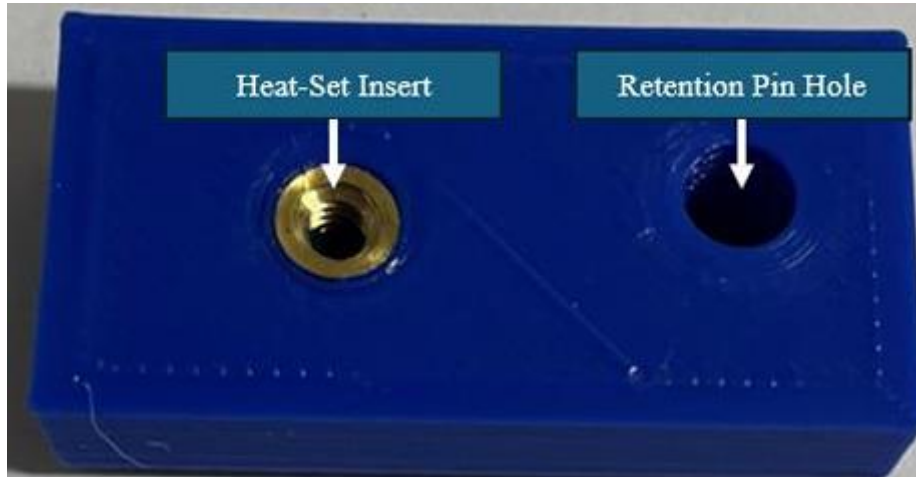
FIG 4: Example of heat-set insert in a 3D printed part reproduced from [25]
