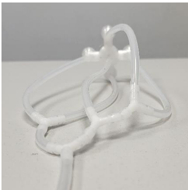
FIG 50 All vacuum inputs connected using splitters
